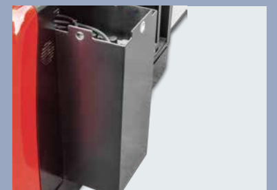
Battery side roll out
