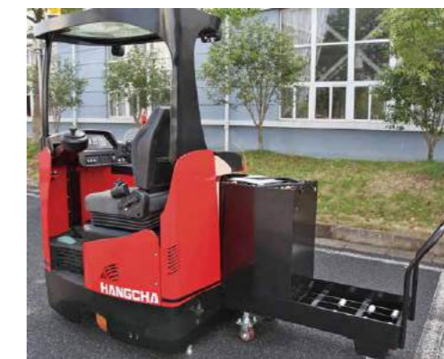
Standard configuration: Battery side roll-out + trolley(optional)
